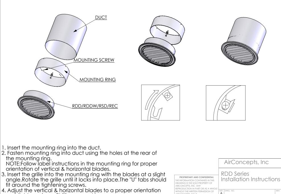
and tighten using a Phillips screw driver.
