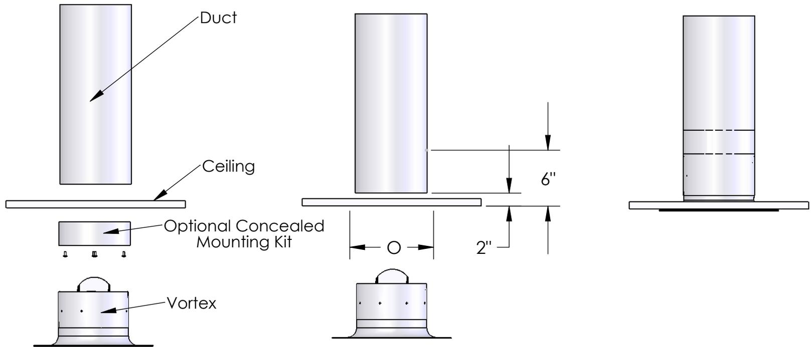
1. Insert the mounting ring into the duct 6" from face of ceiling.
